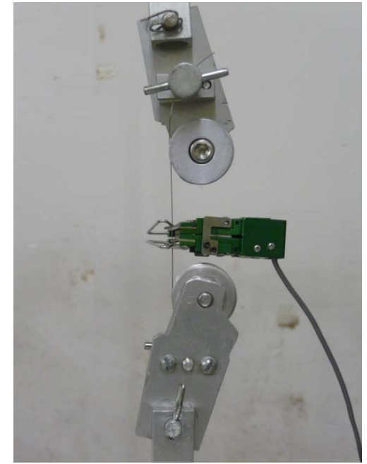
Tensile testing of stainless steel wire
