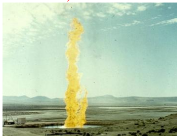
Fire on an unconfined pool of LNG spreading on water 16
