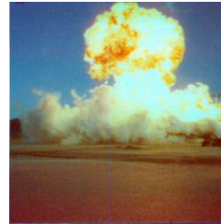
Result of early (accidental) ignition of vapor cloud formed in FALCON Test # 5
