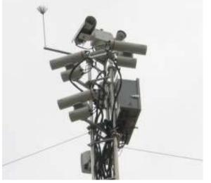
Cerberus Imaging Head W/ Both Thermal and Day cameras Staring Cameras, Lower ones, Slew camera ctr top
