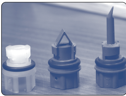
Figure 2 Battery vent caps (from left): OEM, new non-aerobatic, and new aerobic. The government design for the new vent caps used improved technology.
