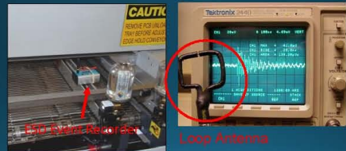
Discharges Recorded as Boards Enter Reflow
