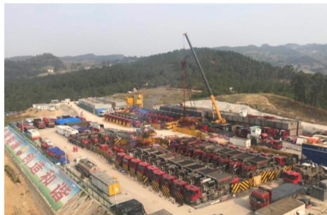
Well factory fracturing with two frac teams
