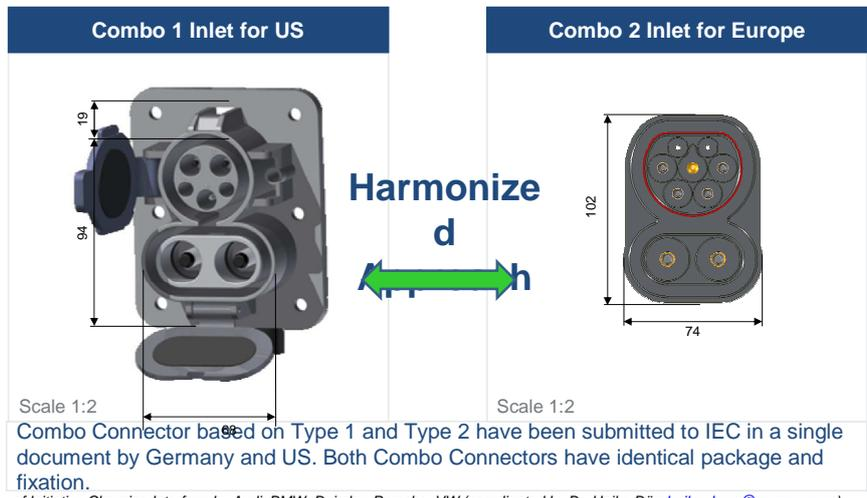
Combo Connector based on Type 1 and Type 2 have been submitted to IEC in a single document by Germany and US. Both Combo Connectors have identical package and fixation.
