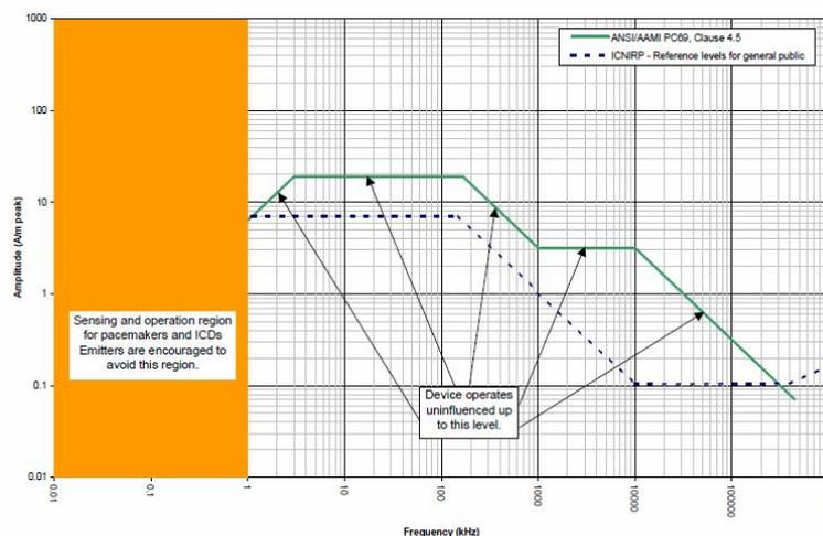
Figure M.2—Magnetic field amplitudes producing test limits
