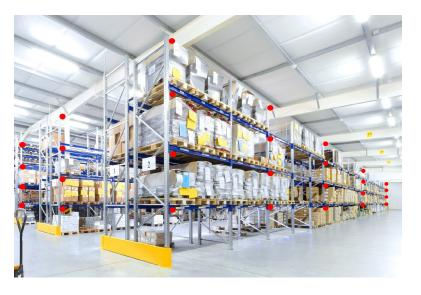
If the ceiling height is 3.6 m or less, position the loggers directly above one another at high, medium and low level -> floor level, one at 1.2 m and one EDLM at 3.0 m
