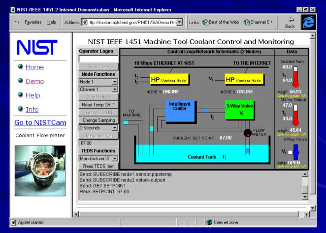
The Java-based remote monitoring and control applet
