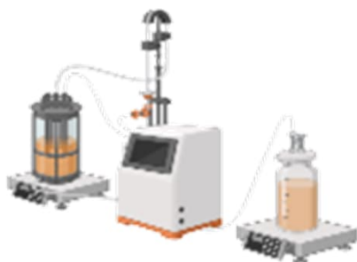
Tangential flow filtration
