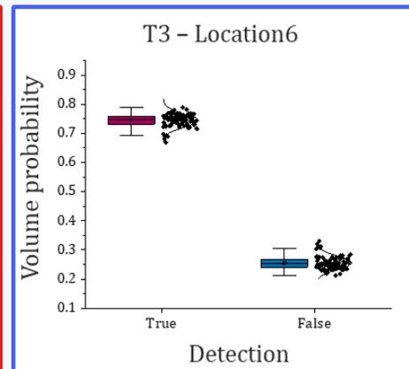
~75% prediction rate for pores larger than 120 micron
