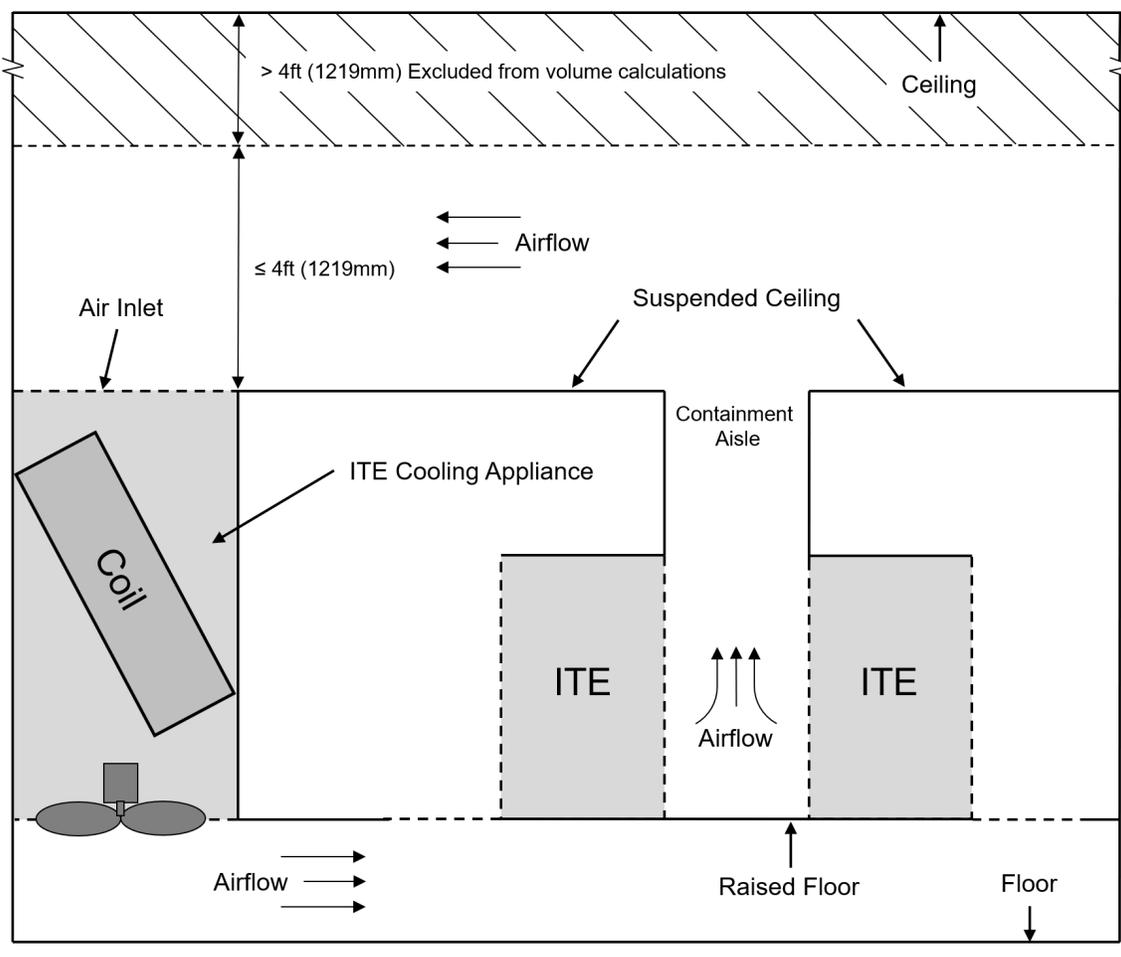
**Figure A7-1 Example elevation view of an *ITE room* for determination of *effective dispersal volume (EDV)*.**
