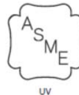
Figure UG-129.1 Official Certification Mark to Denote the American Society of Mechanical Engineers' Standard for Pressure Relief Valves
