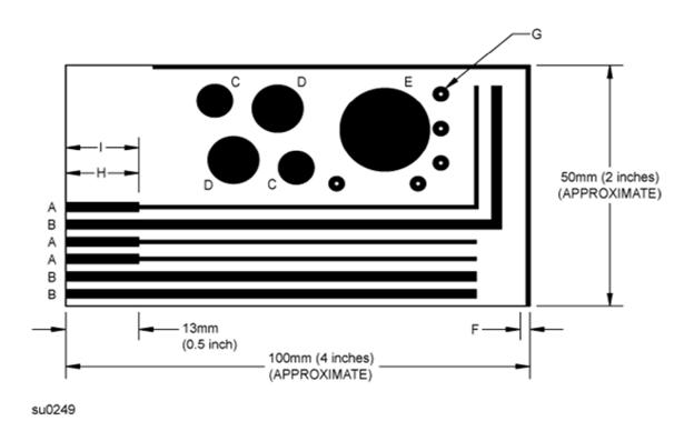
A - Minimum width conductor of configuration specified by the fabricator. See 10.7 and note e.
