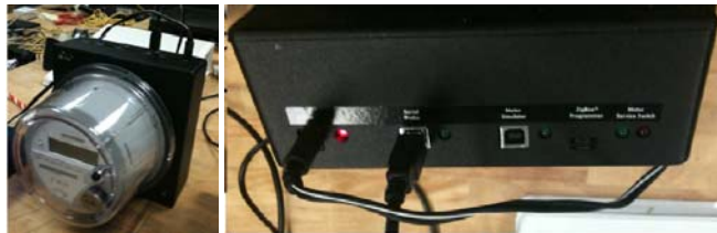
Connectors/connectivity- Zigbee, USB, serial, power, status Allows user to emulate Grid messages/power flow, etc.
