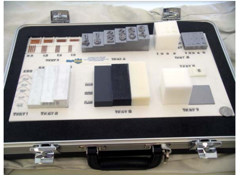
ANSI N42.45 Test Article for CT Security Screening Systems
