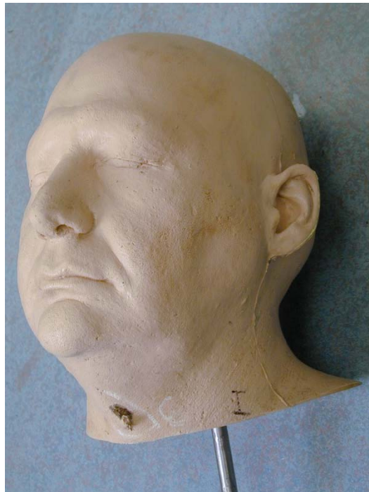
Figure 6 Ironman Silicone “Skin” Over Steel Sphere Head Form
