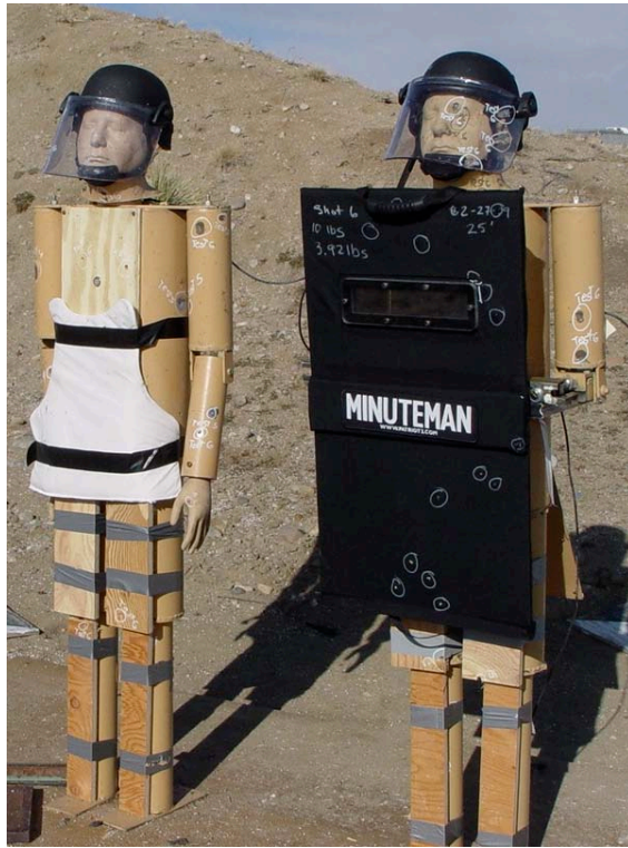
Figure 15 Ironman with Ballistic Vest after Shot 6
