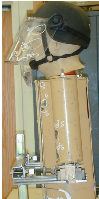
Figure 4 Photo Depicts Roller Bearing Sleeve Fore-Arm System
