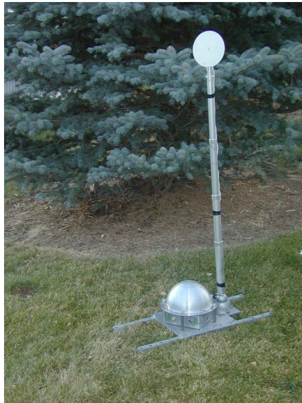
Figure 7 Measure Air blast Remote Station (MARS) Probes
