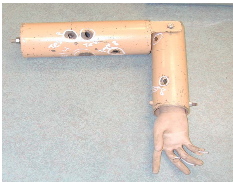
Figure 18 Example Fragmentation Damage to Ironman Arms and Hand Form
