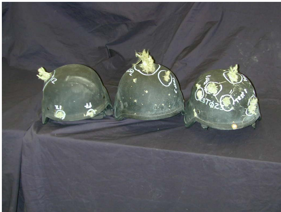
Figure 20 Example Helmet Fragmentation Damage
