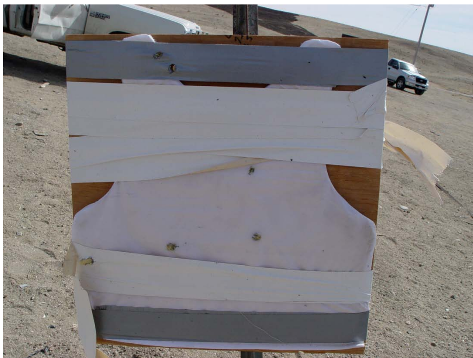
Figure 21 Fragment Impact Points on Ballistic Vest
