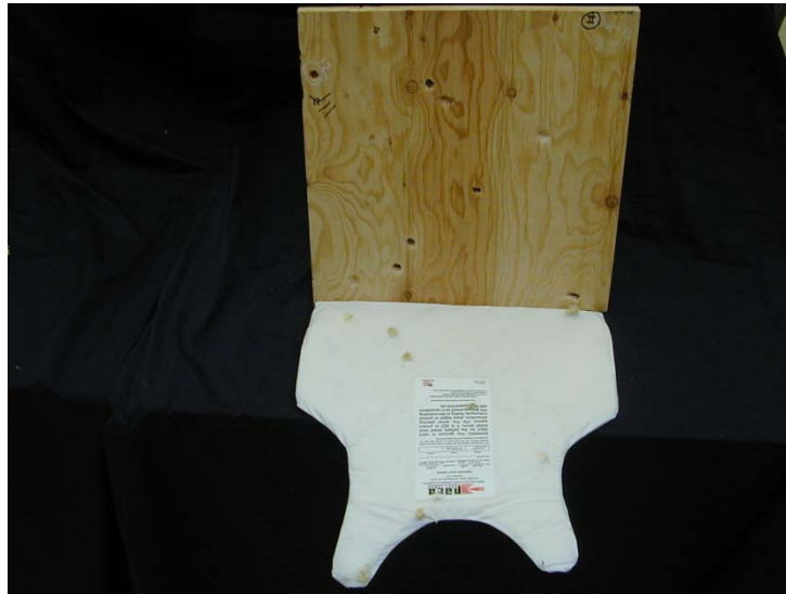
Figure 23 Back of the Ballistic Vest Exhibiting Penetrations
