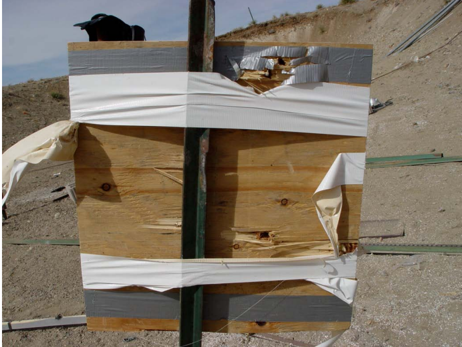
Figure 22 Rear View Exhibiting Penetration of Ballistic Vests and Plywood Panel
