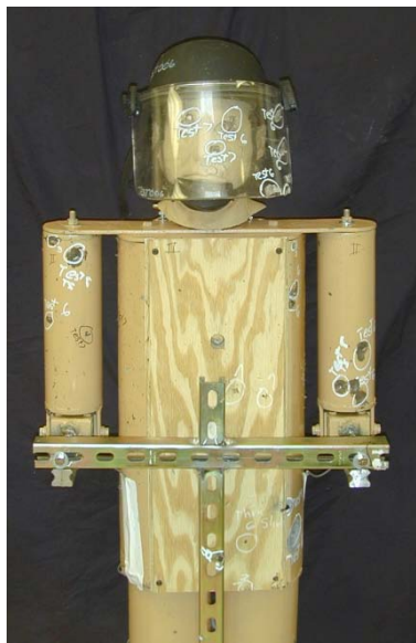
Figure 5 Photo Depicts Ballistic Shield Attachment System
