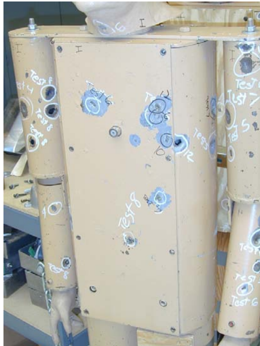
Figure 16 Example General Fragmentation Damage to Ironman
